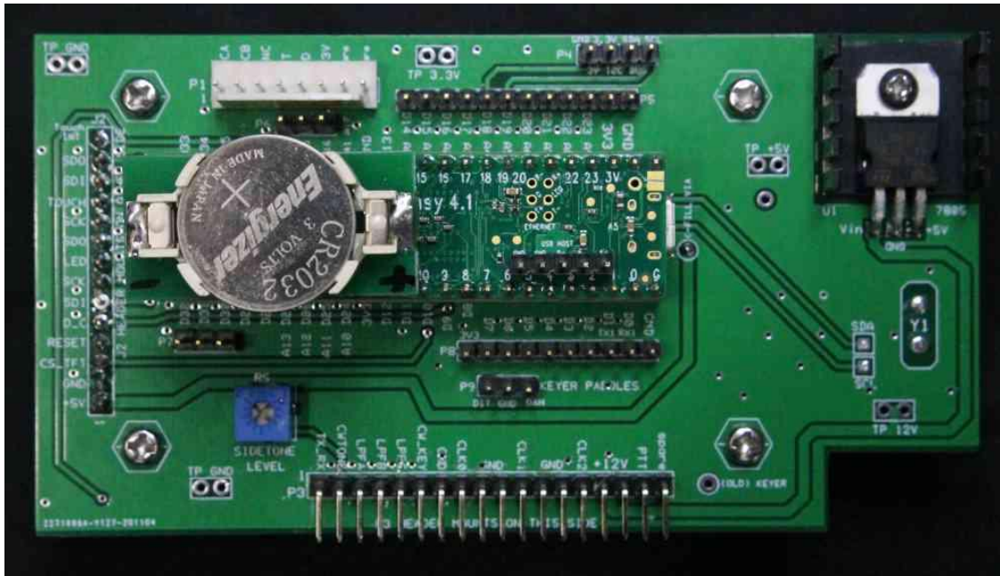
Completed V6 Raduino clone (shown from the rear) ready to plug in and use.
