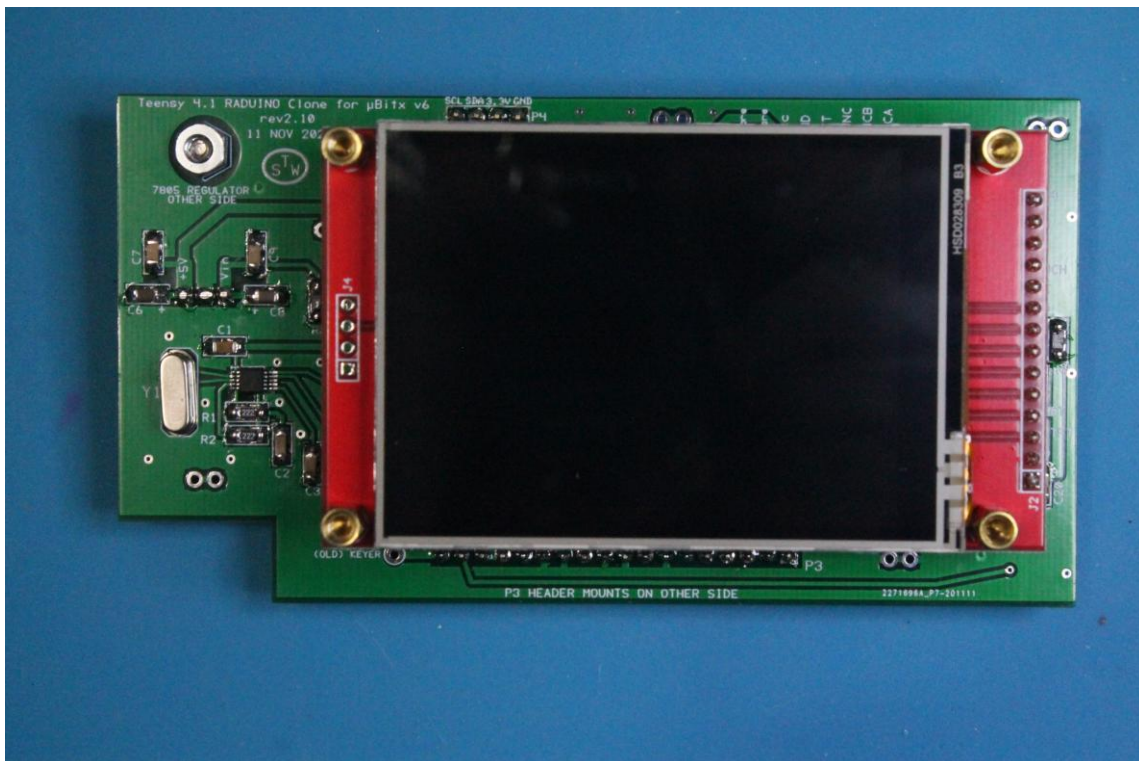
Completed V6 Teensy 4.1 Raduino clone (shown from the front) ready to plug in and use.
