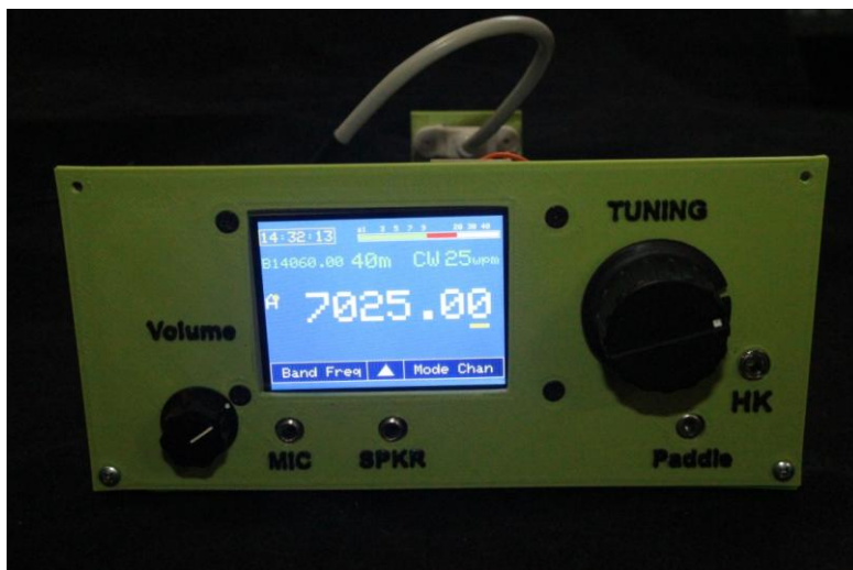
μBITX TSWT4.1 Raduino Clone V2.13 Running on WOEB's test rig.
