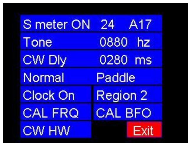
Tone Decoder installed & Selected
