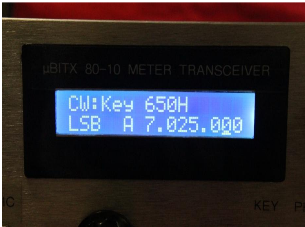
The cursor under the digit can be moved by tapping the encoder button.
