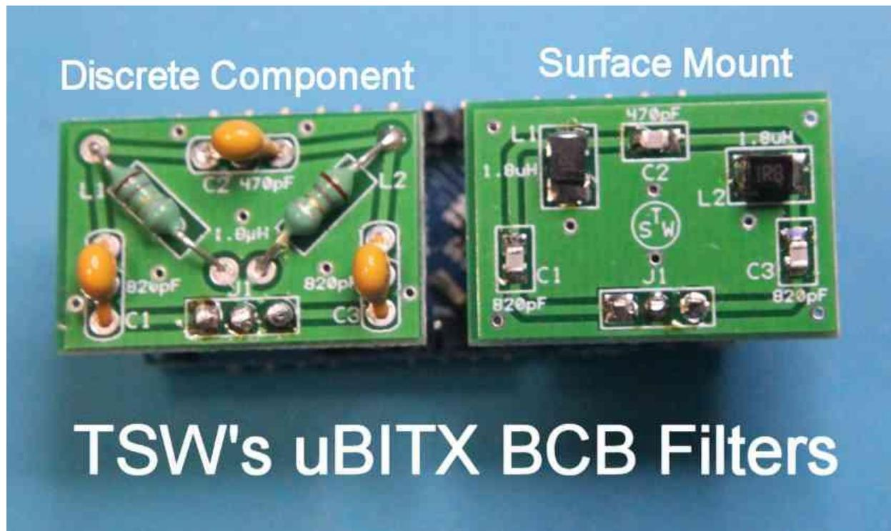
Through hole and Surface mount BCB filters for the  $\mu$ BITX Transceivers.
