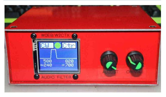
W0EB's build of the filter with the 1.8" Color touch Screen showing the adjustable CW filter. Green dot - CW Zero Beat indicator when incoming tone matches the filter's Center Frequency.
