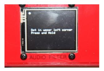
Using a blunt wood or plastic stylus, press and hold the dot in the upper left corner of the screen until the program averages and saves the X-Y coordinates for the upper left corner of the screen and the dot jumps to the lower right corner as in the following image.
