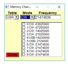
To change Mode, Frequency or both in a given table, click on the check box next to the memory channel you wish to change then click on mode which changes to whichever mode (CW, USB, LSB, SWU or SWL) you want for that channel. Type in the frequency (no decimal point and a leading zero below 10 MHz), hit enter and that memory location is updated to the new mode and frequency. Click on "Close" to close the window.
