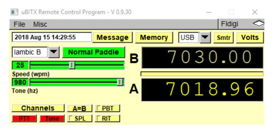
Click on Misc and then click on Configure I/O which will bring up the dialog box where you will see COM ports listed. The COM Port that your uBITX is connected to should appear in the list. Click on it and click the CLOSE button that will appear at the bottom of the list once the port is selected.
